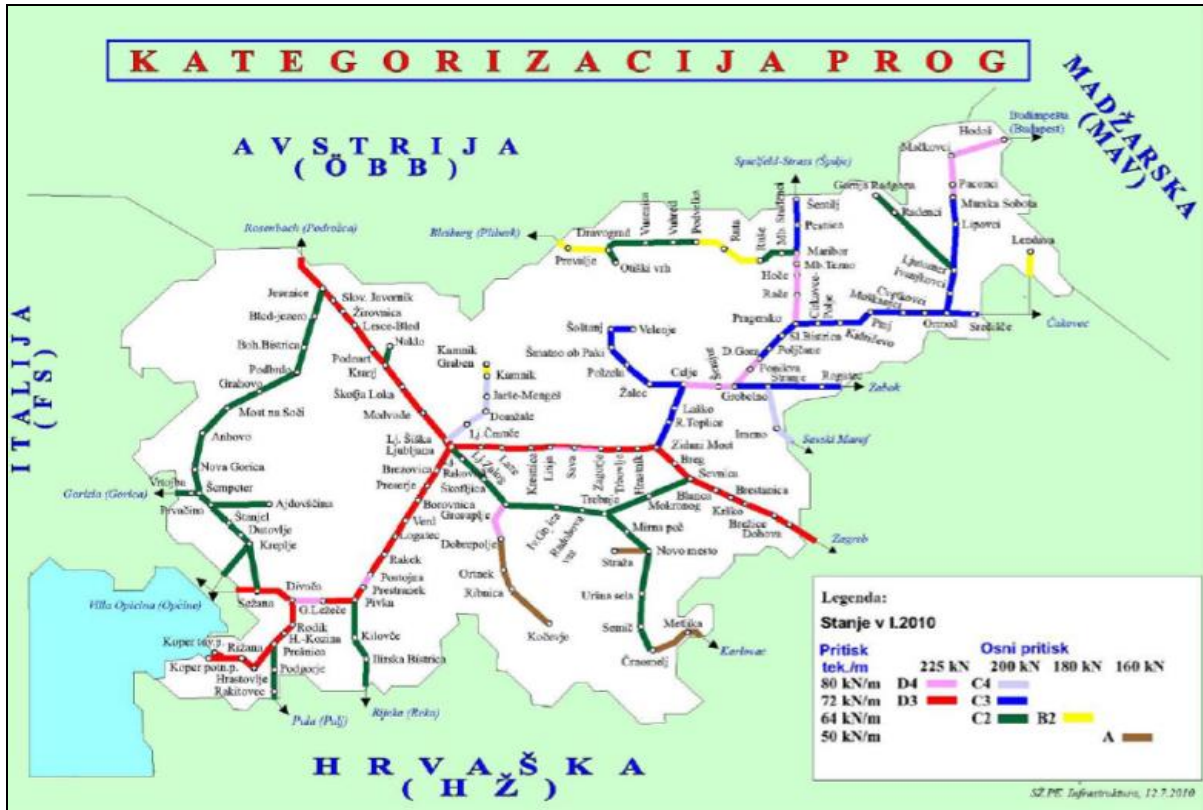
Figure 61 Load-bearing capacity of railway tracks
